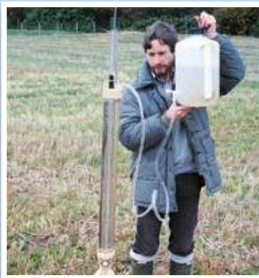
2) Install Permeameter and fill with water
