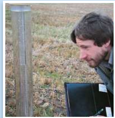
3) Record changing water level and calculate results
