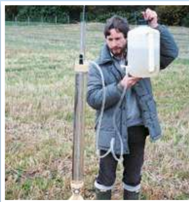
2) Install Permeameter and fill with water
