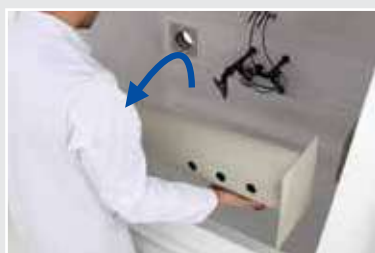
1 The air system collection tube is easily removed.
